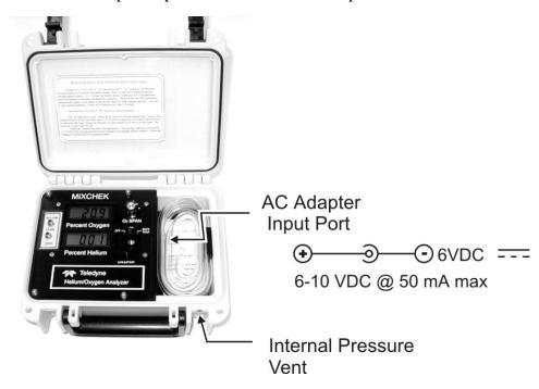
Figure 2-5: Power Adapter Port (Portable Model)
