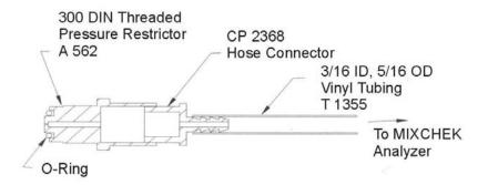
Figure 3-1: Typical Setup Flow Diagram
