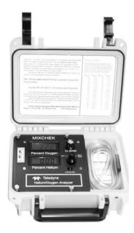
Figure 1-2: MIXCHEK—Portable Configuration
