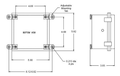
Figure 2-1: Mounting Dimensions
