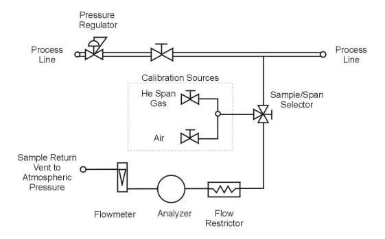
Figure 2-7: Typical Sample System with Provisions for Calibration
